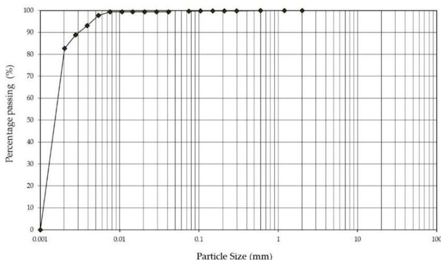
Figure 2. Particle size distribution curve of the WTP sludge.
