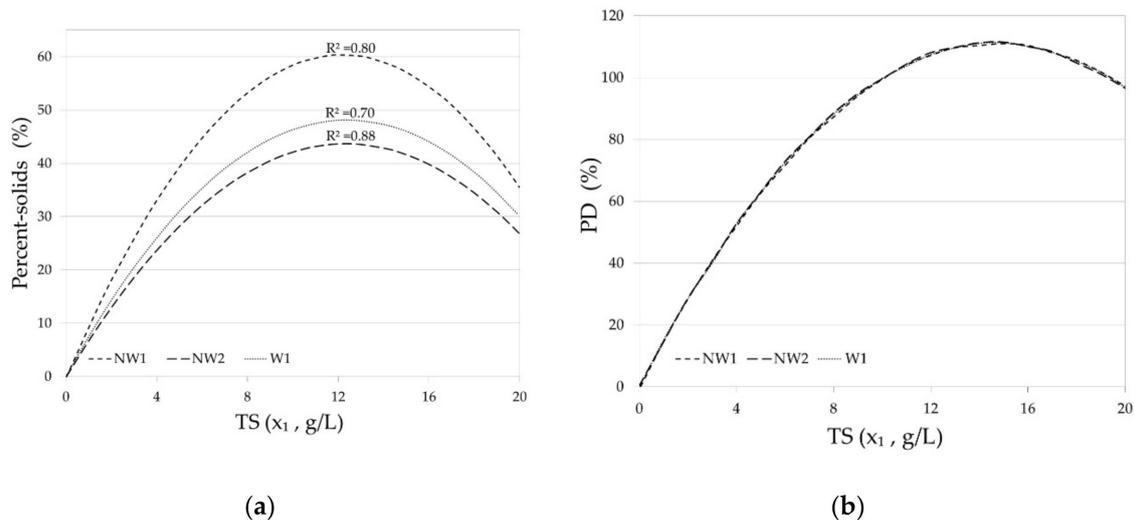
**Figure 9.** Response surfaces of the geotextiles: (a) Percent-solids. (b) Percent Dewatered (PD).
