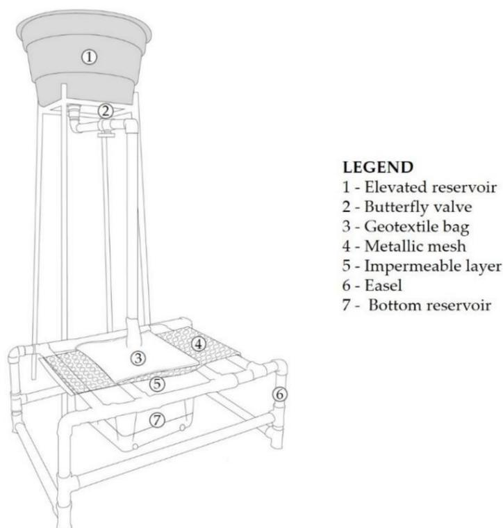
**Figure 3.** Geotextile tube dewatering test scheme.
