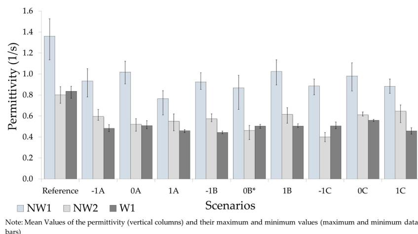
**Figure 11.** Geotextiles permittivity—effects of sludge dewatering.
